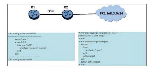
Router R2 advertises the network 192.168.3.0/24 to router R1 via OSPF. A route policy has been constructed to discard the route on router R1; however, it is not working. What is the problem?
