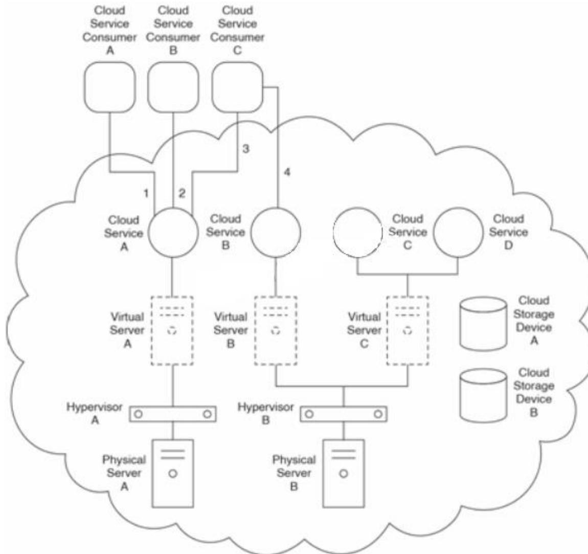
Cloud Service Consumers A, B and C simultaneously access Cloud Service A. Cloud Service Consumer C receives a runtime exception and its request for access is rejected. It is determined that Cloud Service Consumer C attempted to upload a large amount of input data for Cloud Service A, which exceeded the bandwidth threshold of the virtual network. The cloud architecture needs to be improved to avoid this from happening again.
