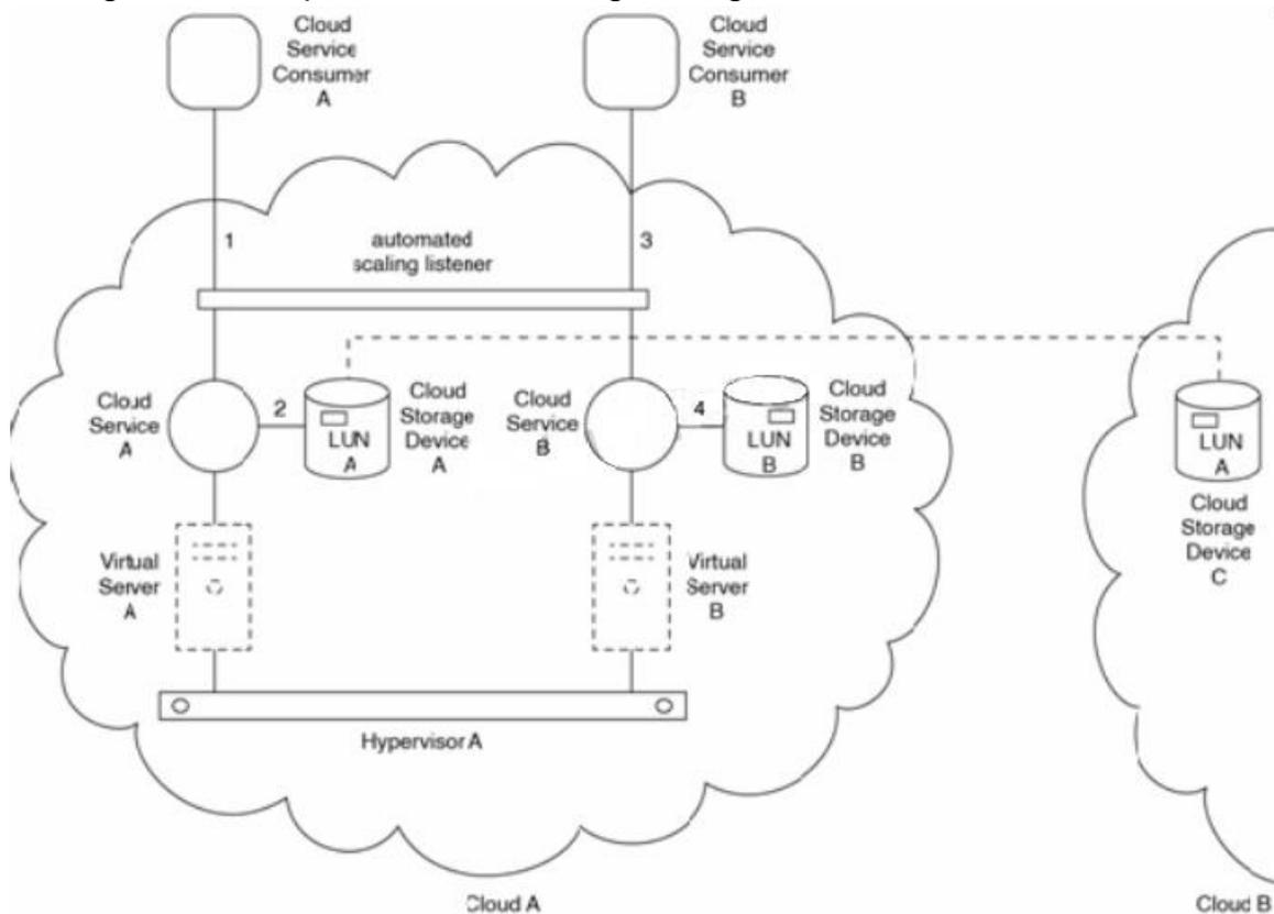
Cloud Service Consumer A issues a request to Cloud Service A (1). To process the request, Cloud Service A accesses LUN A on Cloud Storage Device A (2). Cloud Service Consumer B issues a request to Cloud Service B (3). To process the request, Cloud Service B accesses LUN B on Cloud Storage Device B (4).
